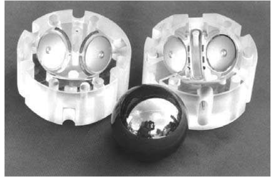
Figure 2. GP-B Gyroscope; clearly seen are the suspension electrodes and spin-up channel.
